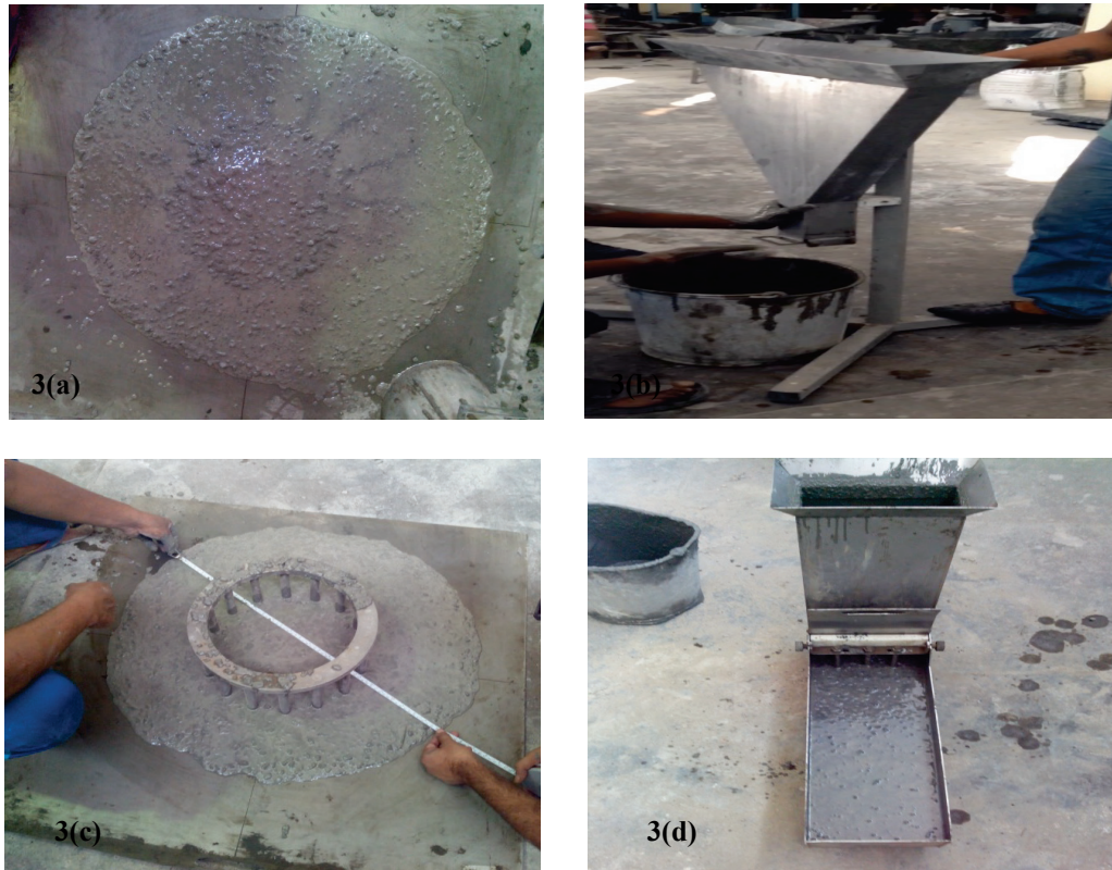
Fig. 3 - (a) Slump flow test, (b) V-funnel test, (c) J- ring test, (d) L-box test
