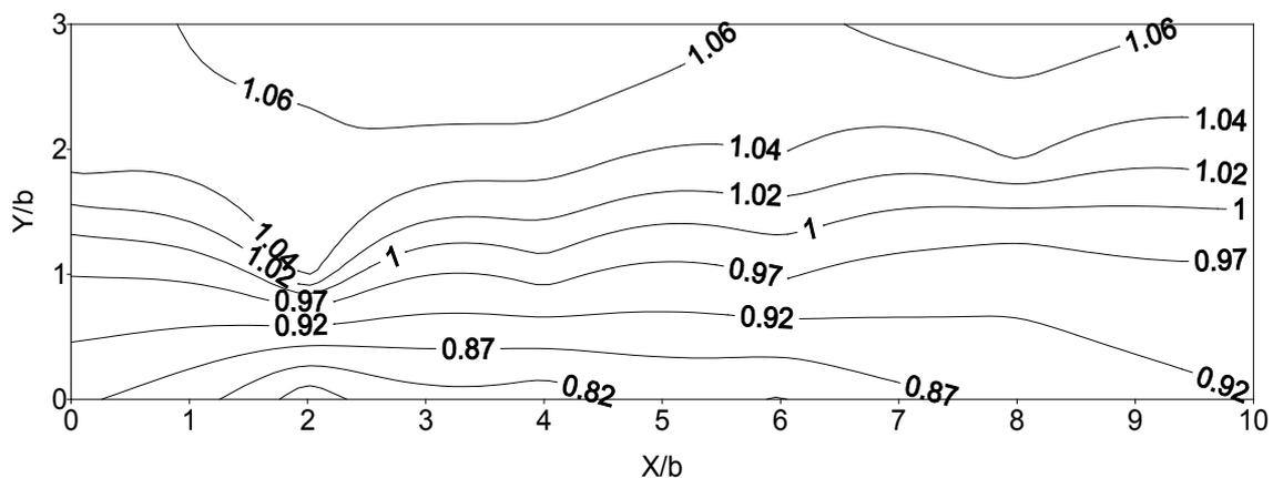
Fig. 5(b) Contour of interference factor for  $H_r = 0.5$
