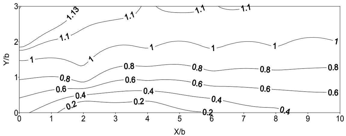
**Fig. 5(e) Contour of interference factor for  $H_r = 1.5$**
