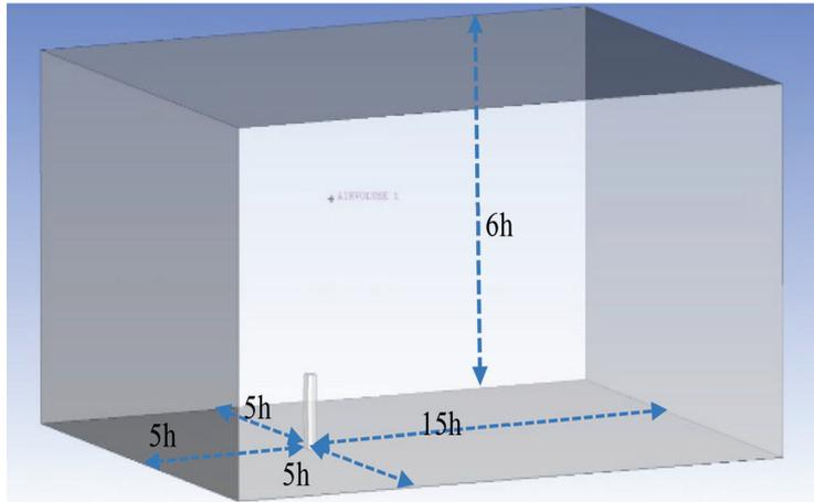
**Fig.1- Computational domain for numerical simulation**
