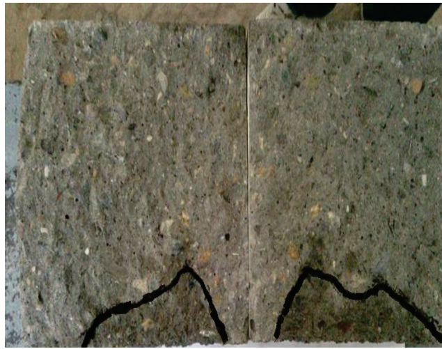
Fig.-3: Water penetration front in one of the water permeability tests
