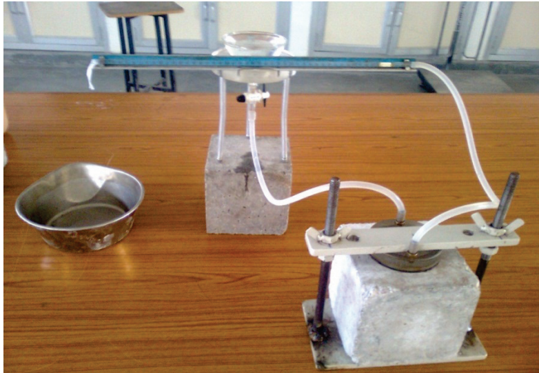
Fig.-2: Test setup for the initial surface absorption test
