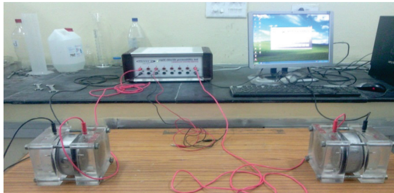
Fig.-5: Test setup for the rapid chloride penetrability test
