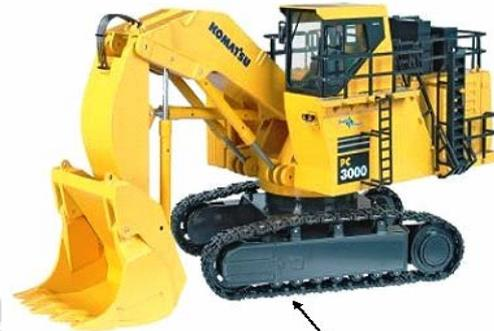
Boden Plate L 800 Excavator PC3000
