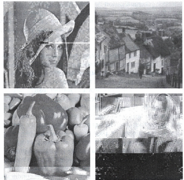
Fig. 2. Distorted image samples showing different artifacts: “Lena” with blocking, “Goldhill” with blur in 8 \times 8 blocks (top); “Pepper” with ringing and intensity masking, “Barbara” with extreme artifacts (bottom).
