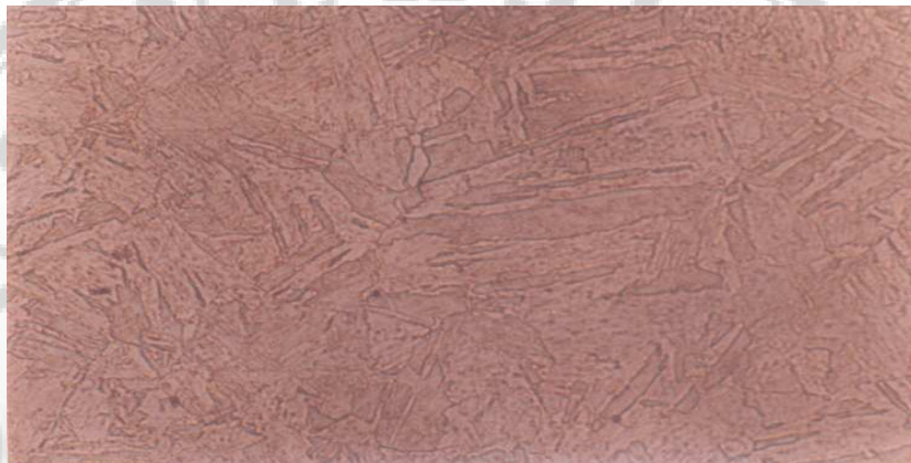
Gambar 3 Struktur Mikro Material Corrax Proses Nitrocarburizing Tanpa Aging Pembesaran 400x
