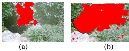
Figure 6. Water segmentation by polarization degree (left) and by Polarization phase(right), water detection is shown in red [8]
