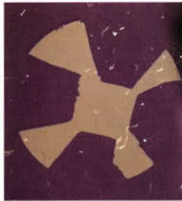
Figure 9: Thin film of copper deposited onto silicon chip.
