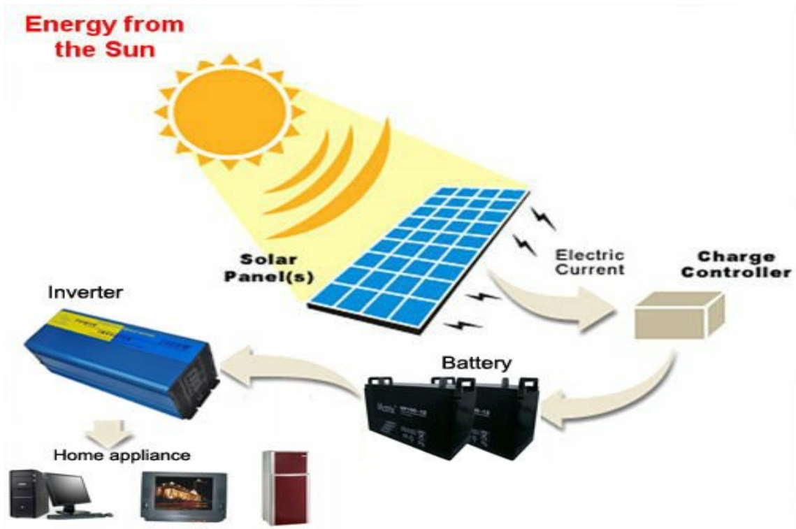
Figure 3.5: The above figure is how solar energy is converted to usable electricity (7)
