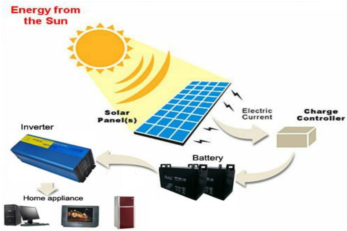
Figure 3.2: How solar energy is converted to a desirable DC voltage and current (4)
