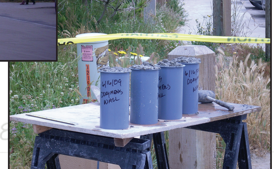
Concrete samples from the pour are tested.
