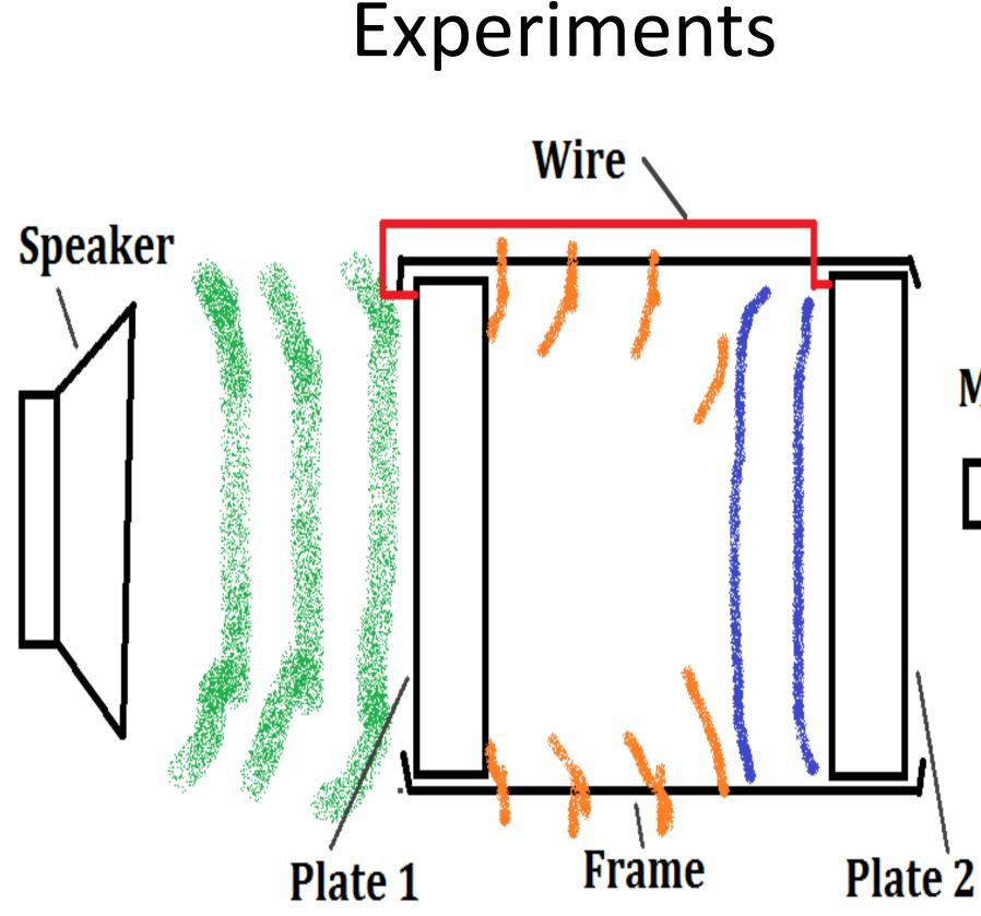
A microphone was used to collect sound waves which passed through the plates in order to determine the effectiveness of the sound damping. The plates were wired so as to separately test the piezoelectric effect (sound absorption) and the converse effect (production of the new wave), and isolate these from other effects which may have contributed to noise reduction. Sound frequencies from 100 to 2000 Hz were tested.
