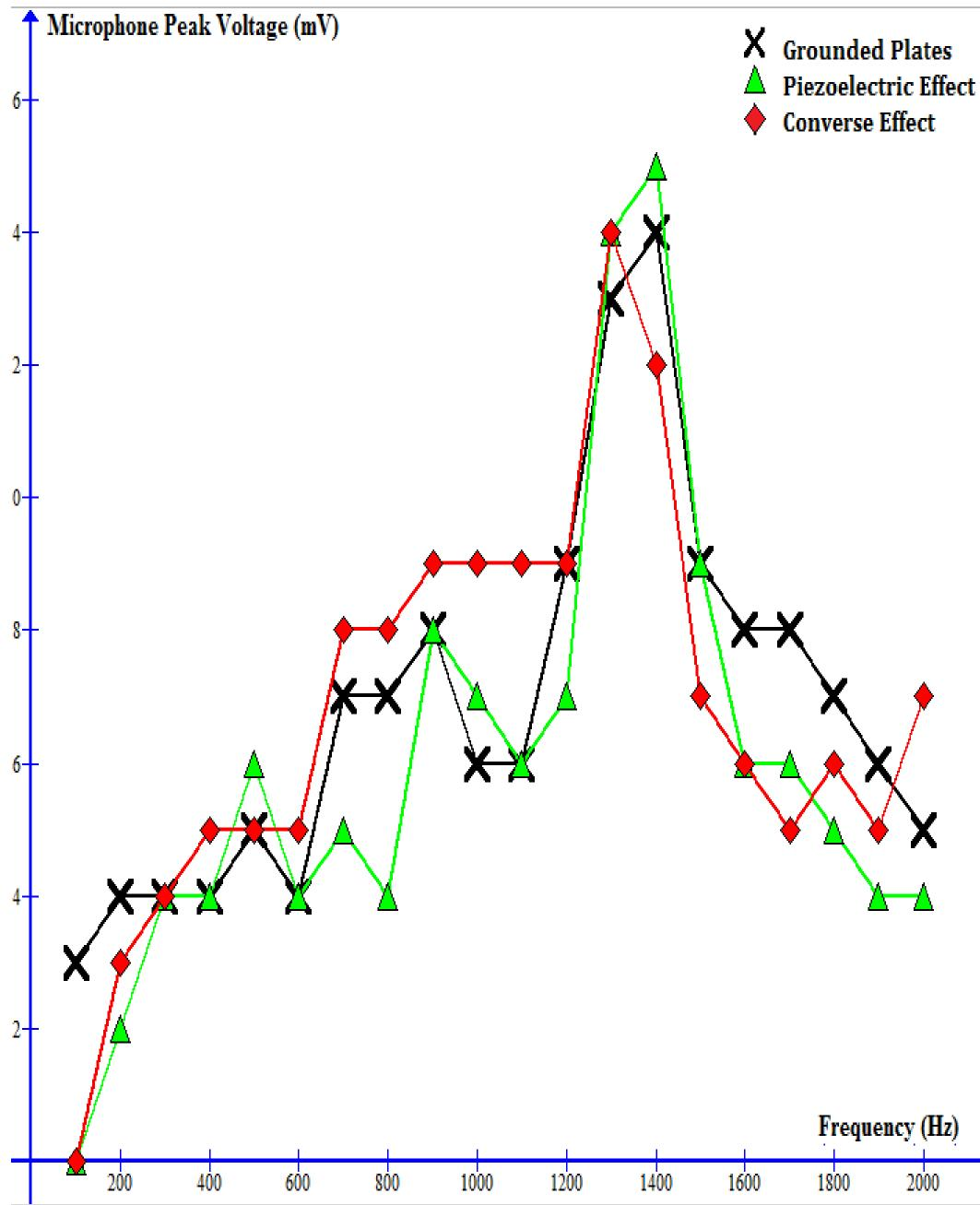
The signal received by the microphone while testing the piezoelectric effect was generally smaller than when the plates were grounded, as expected.
