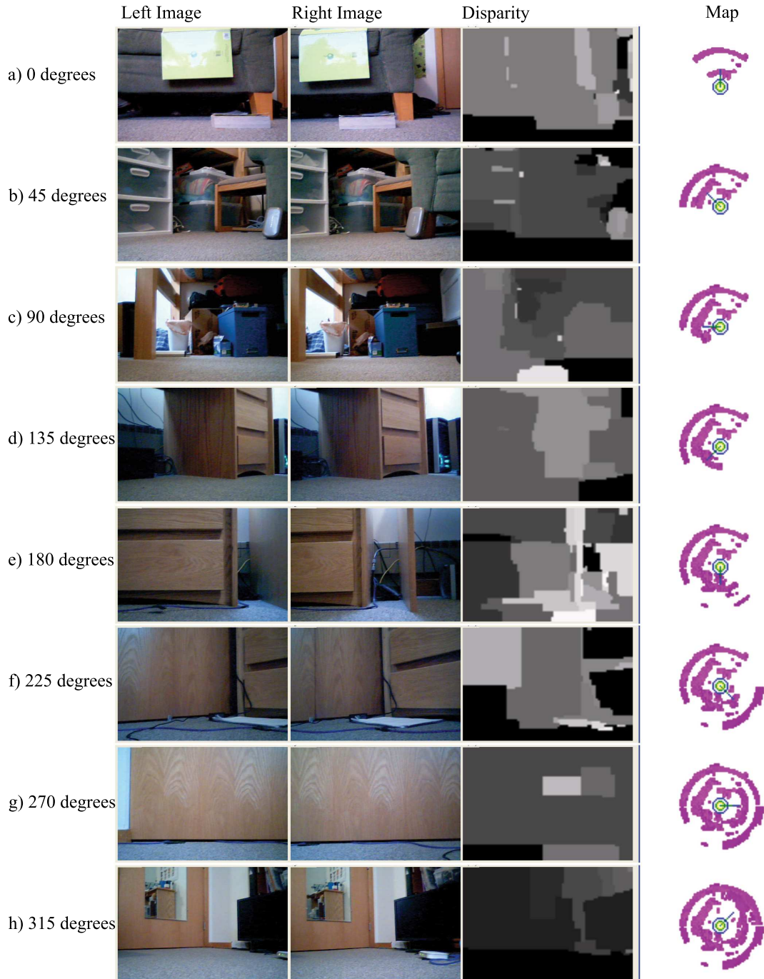
Figure 7: Real life mapping using stereoscopic imaging. The images show the left and right cameras and their combined disparity map. Robot manually rotated around fixed point to scan room and generate initial map. The last image is a top-down image of the robot's internal map. Filled pixels represent blocks (compiled over all height layers of the map) that are filled. The green and blue arrows represent the robot's actual location and the robot's perceived location respectively.
