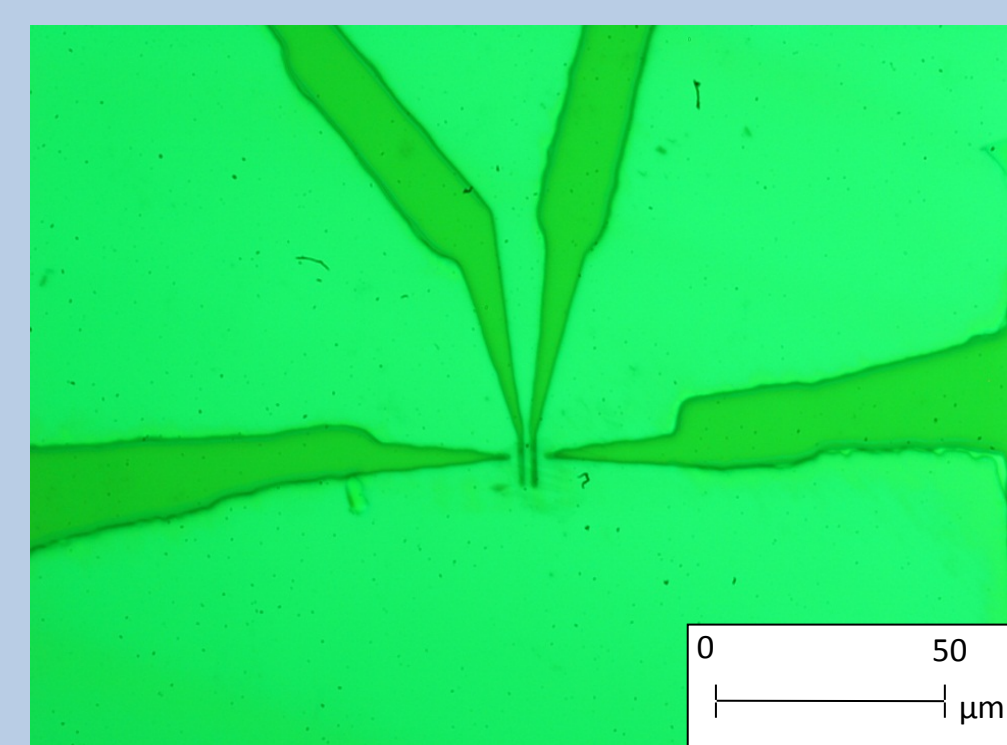
Figure 8. Photolithography prepares patterns that will become circuit leads.
