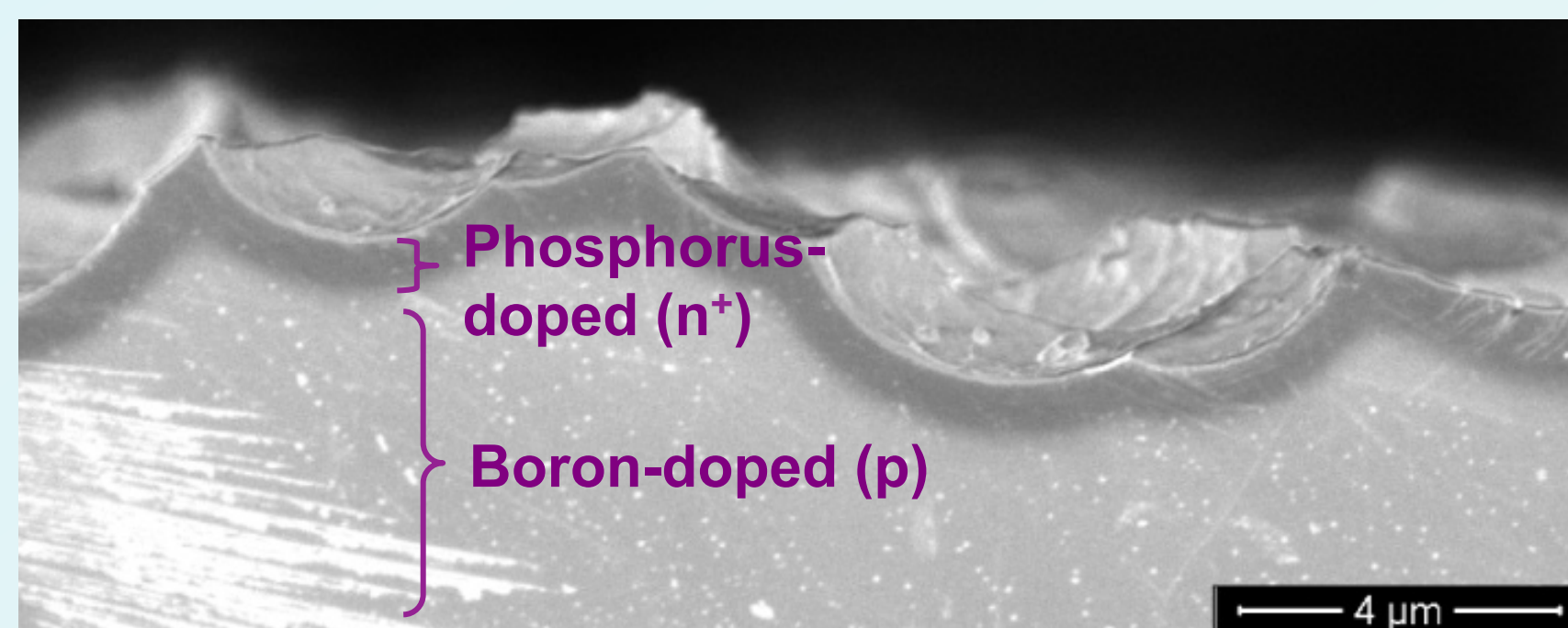
Figure 2. Cross-sectional image of textured surface, obtained using scanning electron microscopy.
