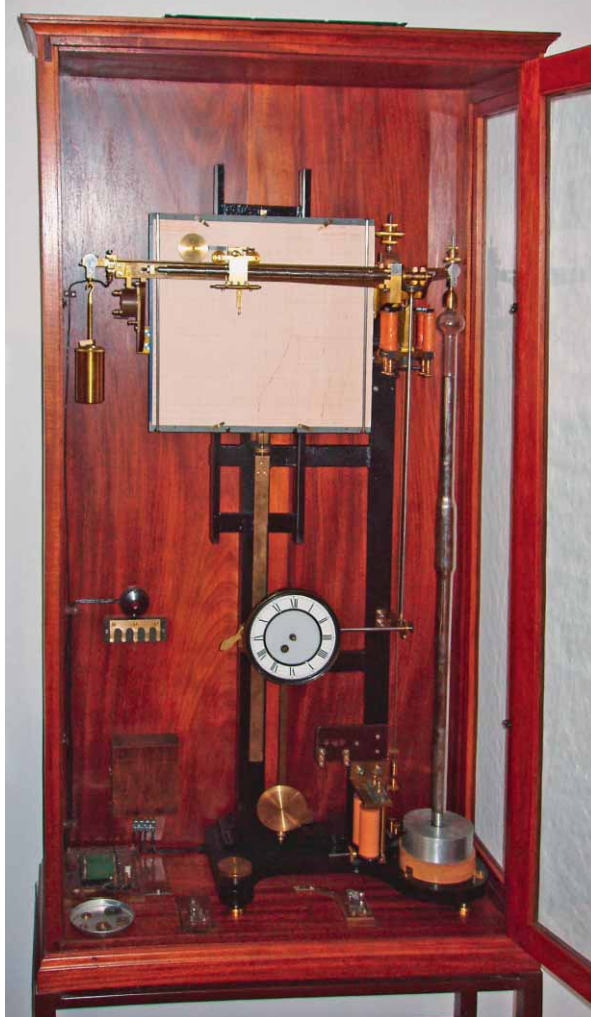
Figure 5. Barograph Sprung-Fuess, installed by Mohorovičić at the Meteorological Observatory in Zagreb in 1903. Among other phenomena, this instrument recorded the passage of atmospheric gravity waves caused by the fall of Siberian meteor in 1908.
