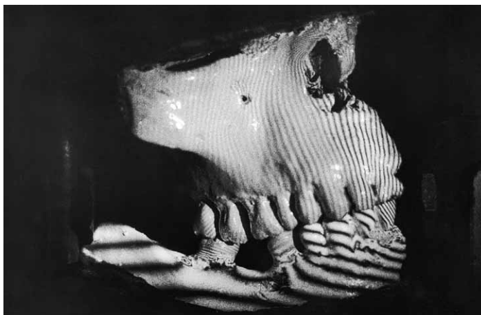
Fig. 2. Interferogram of a preparation with load difference of 10 kP (65 and 75 kP).
