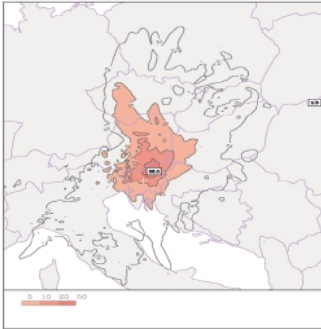
Figure 3. Maximum values of pollution with \text{SO}_2 at 850 hPa from the TEŠ for the period from 1.12.1999 to 29.2.2000 (not necessarily at all points simultaneously!). Gray isolines encircle those areas with more than 2 \mu\text{g}/\text{m}^3 , while the darker area shows where 5 \mu\text{g}/\text{m}^3 was exceeded at least once in the 3-month period.
