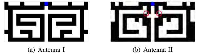
Fig. 9. Sample antennas without and with point crossing. Note that the blue cell and red circles highlight the feed point, and the point crossing junctions, respectively.
