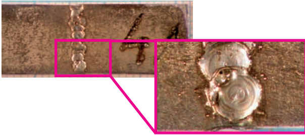
Slika 3. Zavar TIG-postupkom odljevka Co-Cr (I-Bond NF) legure Figure 3 Co-Cr alloy (I-Bond NF) TIG welding
