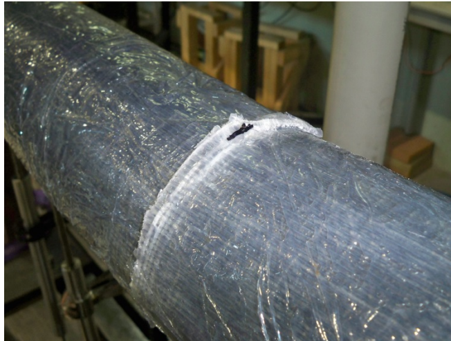
Figure 11: Typical failure mode of the FRP sections (Concept 2) in the compression zone, shown for Set 2
