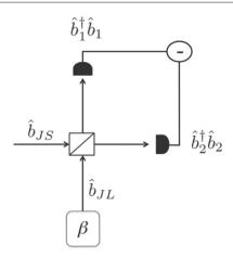
**Figure 5.** Schematic of a homodyne detection to make a quadrature measurement. The signal mode  $\hat{b}_{J,S}$  is combined with the local oscillator mode  $\hat{b}_{J,L}$  and then an intensity measurement is performed. Taking the difference of the two measurements gives an output that is directly proportional to the desired quadrature.
