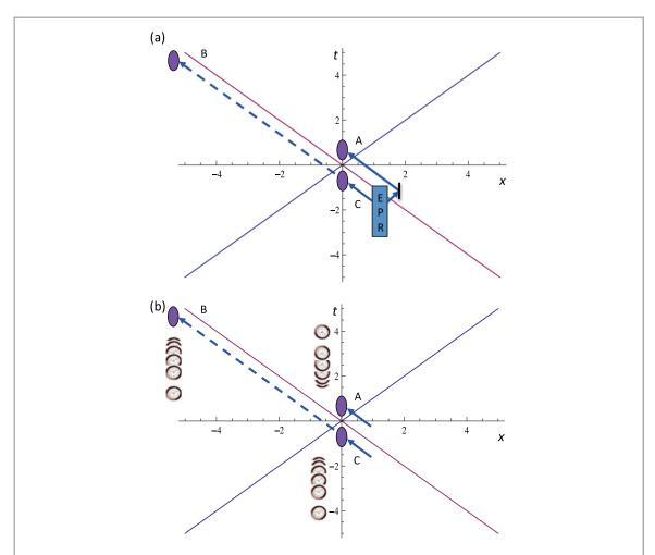
**Figure 3.** Space—time diagram representation of (a) standard continuous variable quantum key distribution and (b) quantum key distribution without sending a quantum signal. The points A and C lie in Alice's station while point B lies in Bob's station. In both cases no measurement is made at point C when the QKD protocol is being enacted. The unequally spaced clocks in (b) represent the energy scaled homodyne detection.
