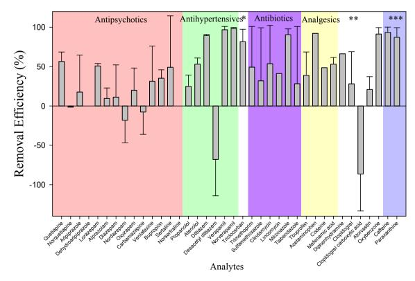
**Fig. 3.** Average removal efficiency ( $\% \pm$  StDev) of PPCPs from STP<sub>U</sub> and STP<sub>M</sub>. \*antimicrobial; \*\*antihistamine (diphenhydramine), antiplatelet (clopidogrel and its metabolite clopidogrel carboxylic acid), hypercholesteremic (Atorvastin), and UV-filter (oxybenzone); \*\*\*stimulant (caffeine and its metabolite paraxanthine).
