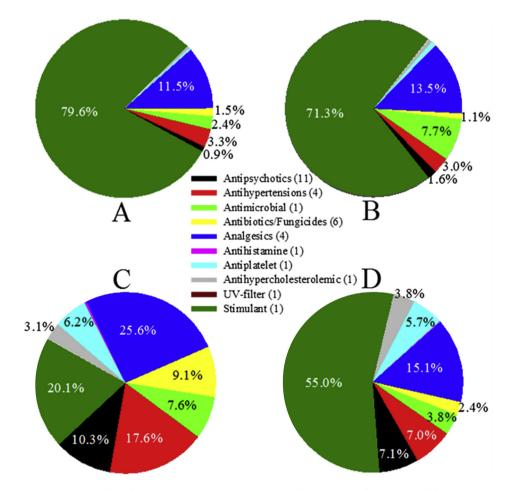
Fig. 2. Percentage composition profiles of selected PPCPs in wastewater. A: STP<sub>U</sub> influent; B: STP<sub>M</sub> influent; C: STP<sub>U</sub> effluent; and D: STP<sub>M</sub> effluent.
