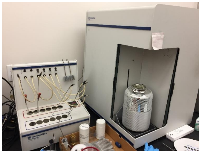
FIGURE 3.5 – BET surface analyzer used for surface area and pore size analysis
