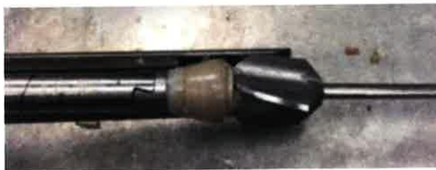
Figure 29: The peek bearing sustained substantial wear throughout the two rounds of testing (.8mm of material lost). It is suggested that if modifications to this design are performed, reversing the material of the bearing and follower sleeve may be more advantageous to reducing the amount of wear to the components.
