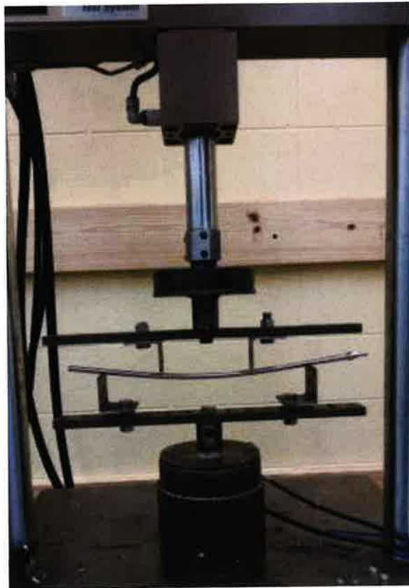
Figure 37: Shown above is the experimental setup for generating a four point bending load on the Stryker flexible reaming shaft. This method of loading allowed the team to isolate the bending stiffness of the flexible shaft (Eqn. 6-8). In order to develop the flexible follower sleeve, this experiment was replicated in SolidWorks 2015 Academic Edition.
