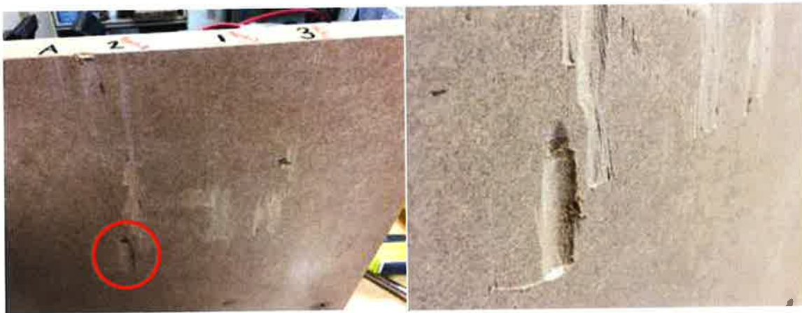
Figure 23: Circled above is the location of deflection reaming using the 14mm reamer head. Only a depth of 2.3mm was achieved from this trial.
