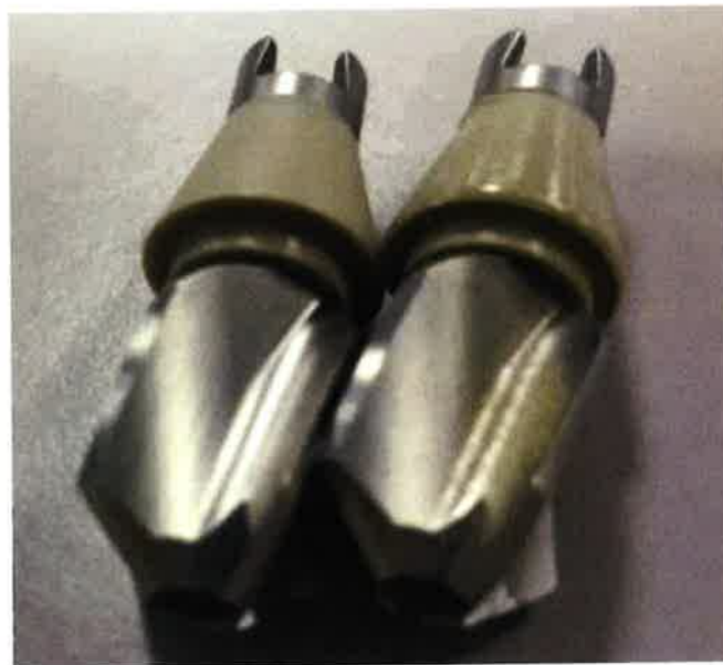
Figure 25: The modified reamer head on the left is unused and shows the amount of wear the reamer used in the sawbones experiment (right) sustained.
