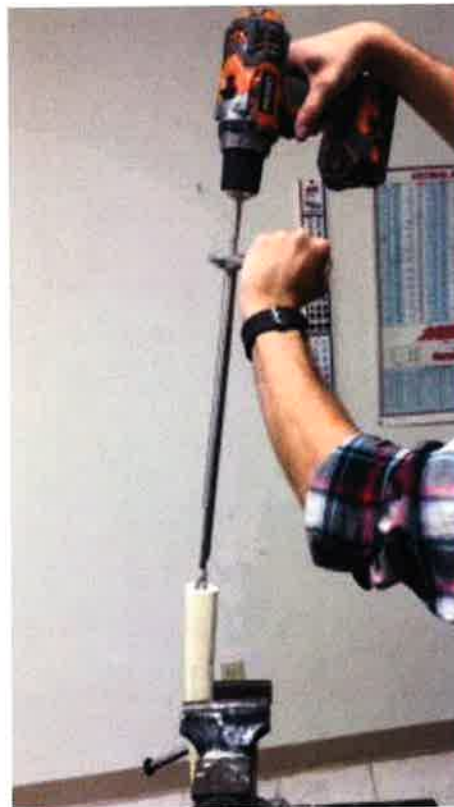
Figure 20: Devicix saw bone test is pictured above.
