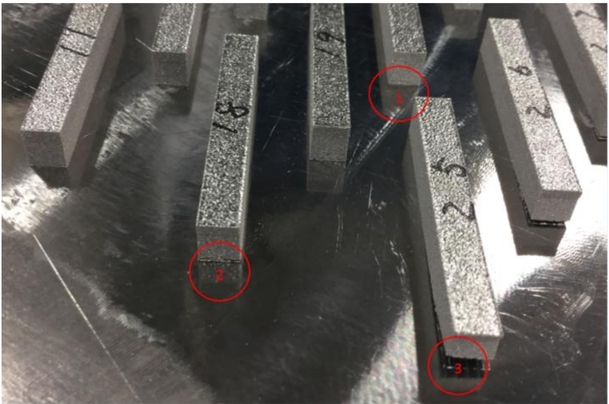
Figure 106 Support structure cracking at the bottom
