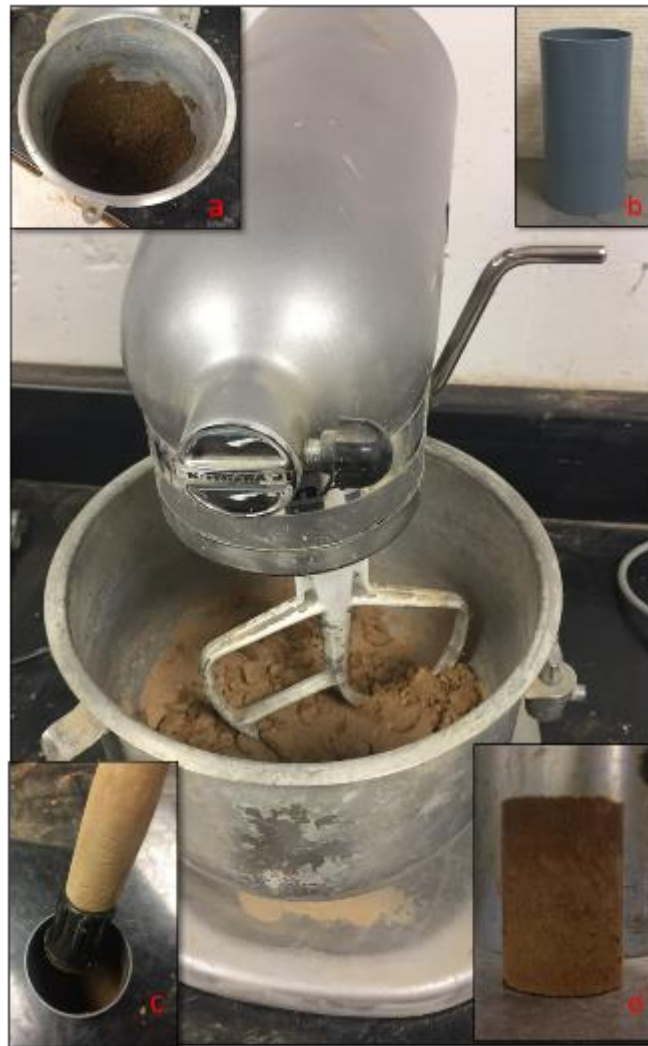
Figure 5-1. Procedure of making S/S specimen
