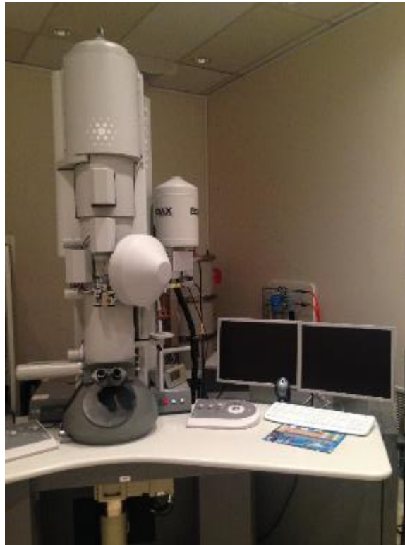
Figure 2-12. FEI Tecnai TEM machine (University of Louisville)
