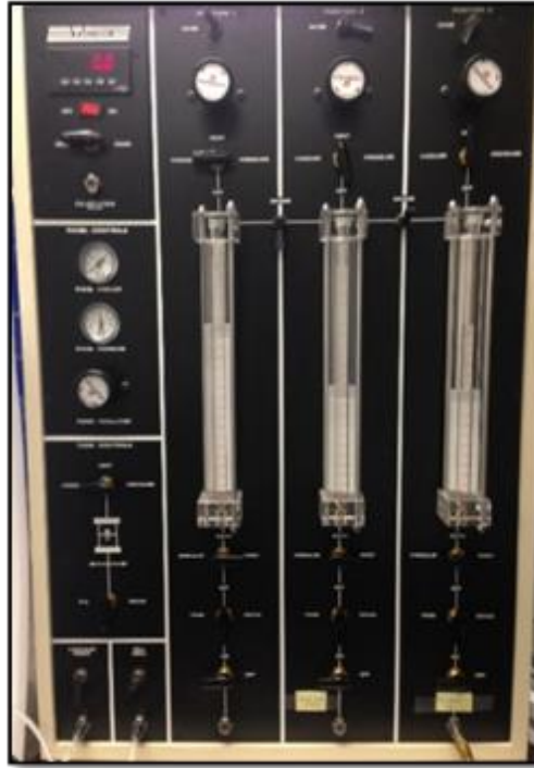
Figure 3-6. Pressure control panel (Trautwein soil testing Co.)
