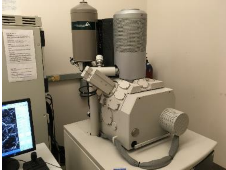
Figure 2-9. SEM machine (University of Louisville)
