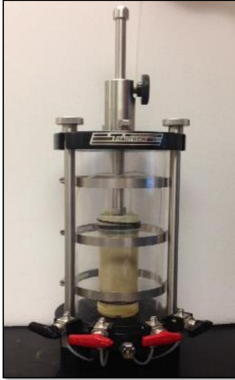
Figure 3-10. The setup of the triaxial cell
