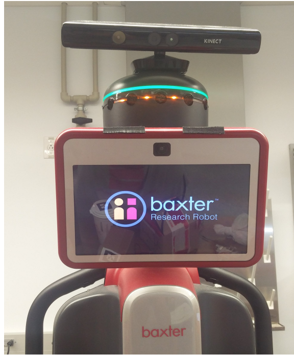
Figure 9: Kinect Camera on Baxter Head
