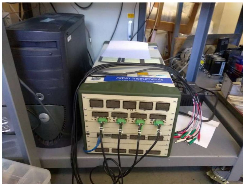
Figure 15. Arbin BT2043™ instrument used for cell cycling.
