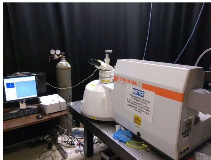
Figure 10. The InVia™ Renishaw Raman microscope used for performing Raman spectra.
