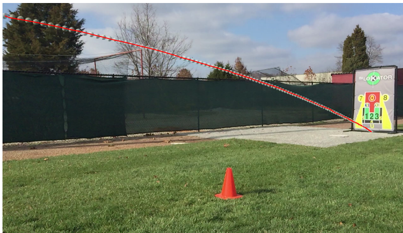
Figure 4.3: A sample pitch from video 5 where the ball was incorrectly classified as hitting the target frame. In this case, the ball bounces off the ground, very close to the target frame.
