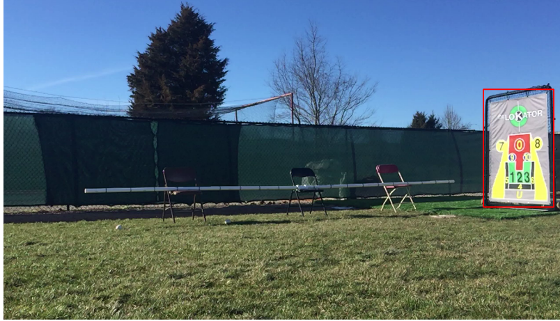
Figure 3.23: Setting used for calibration to learn the pixels spatial resolution at different locations.
