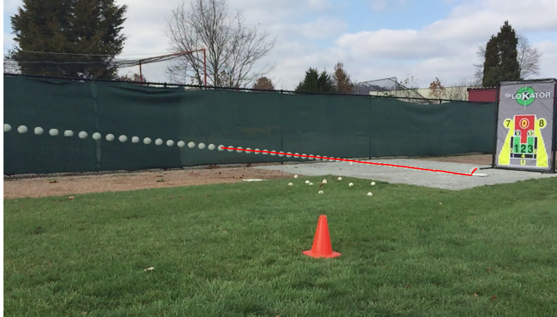
Figure 3.17: An example of a pitch where the Ball bounce off the ground. The algorithm stopped tracking the ball after detecting that it started getting higher.
