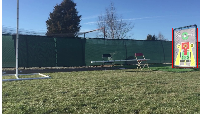
Figure 3.26: Vertical stick used to map a foot length to number of pixels.
