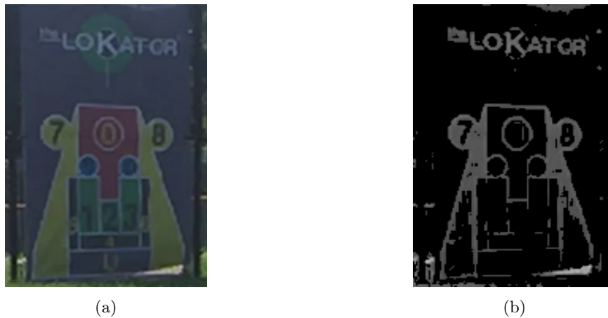
Figure 3.5: (a) Sample image of a target that appears to be too dark. (b) Resulting image after thresholding the one in (a).
