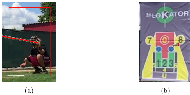
Figure 4.10: Another example of system performance when a catcher is used. (a) Path of the ball and its position when caught by catcher. The red square indicates the position of the target (before it was replaced by the catcher). (b) Replacing the catcher with a virtual target to read the hit zone
