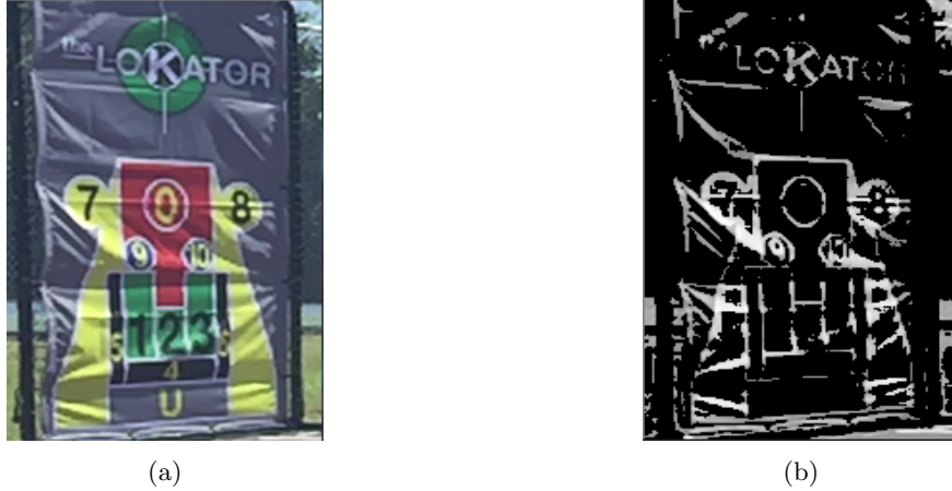
Figure 3.6: (a) Sample image of a target that is not attached properly to the frame. (b) Resulting image after thresholding the one in (a).
