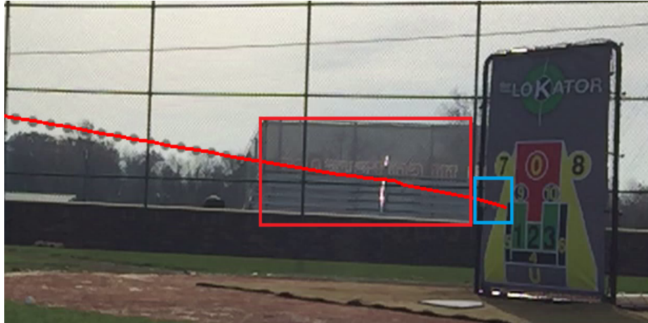
Figure 3.16: The ball is missed in the red box due to the white building (same color as the ball) but Kalman filter predicted smoothly the next locations of the ball. In the blue box, the software was again able to detect the ball twice.
