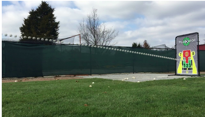
Figure 3.22: Trajectory of a sample pitch. The decrease in the size of the ball as it travels towards the target indicates a decrease in the spatial resolution (as the ball moves farther from the camera).
