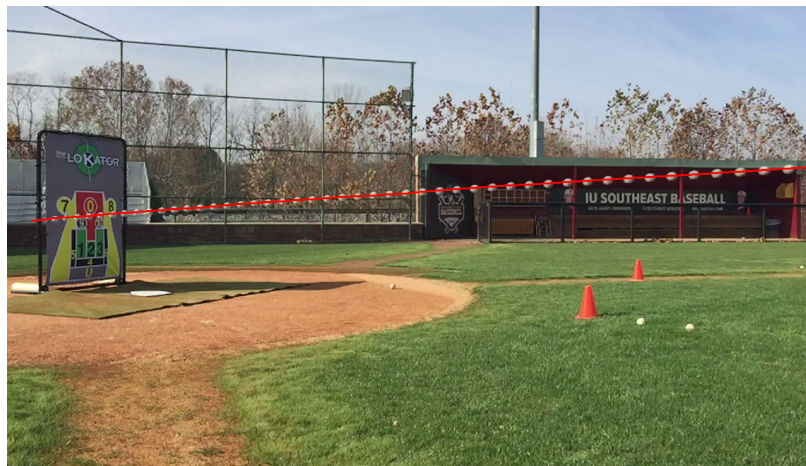
Figure 4.5: Path of the incorrectly detected pitch illustrated in figure 4.4. The ball disappeared between the target and the frame and the software Kalman filter predicted a position that went beyond the target.
