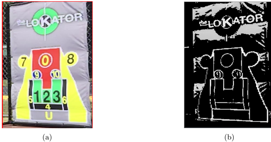
Figure 3.4: (a) Sample image of a target that appears to be too bright. (b) Resulting image after thresholding the one in (a).
