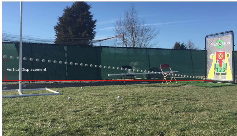
Figure 3.27: Example of calculated vertical displacement. The red lines show the highest and lowest positions of the ball. The obtained distance is equal 1.93 feet which is equal to 0.58 meter.
