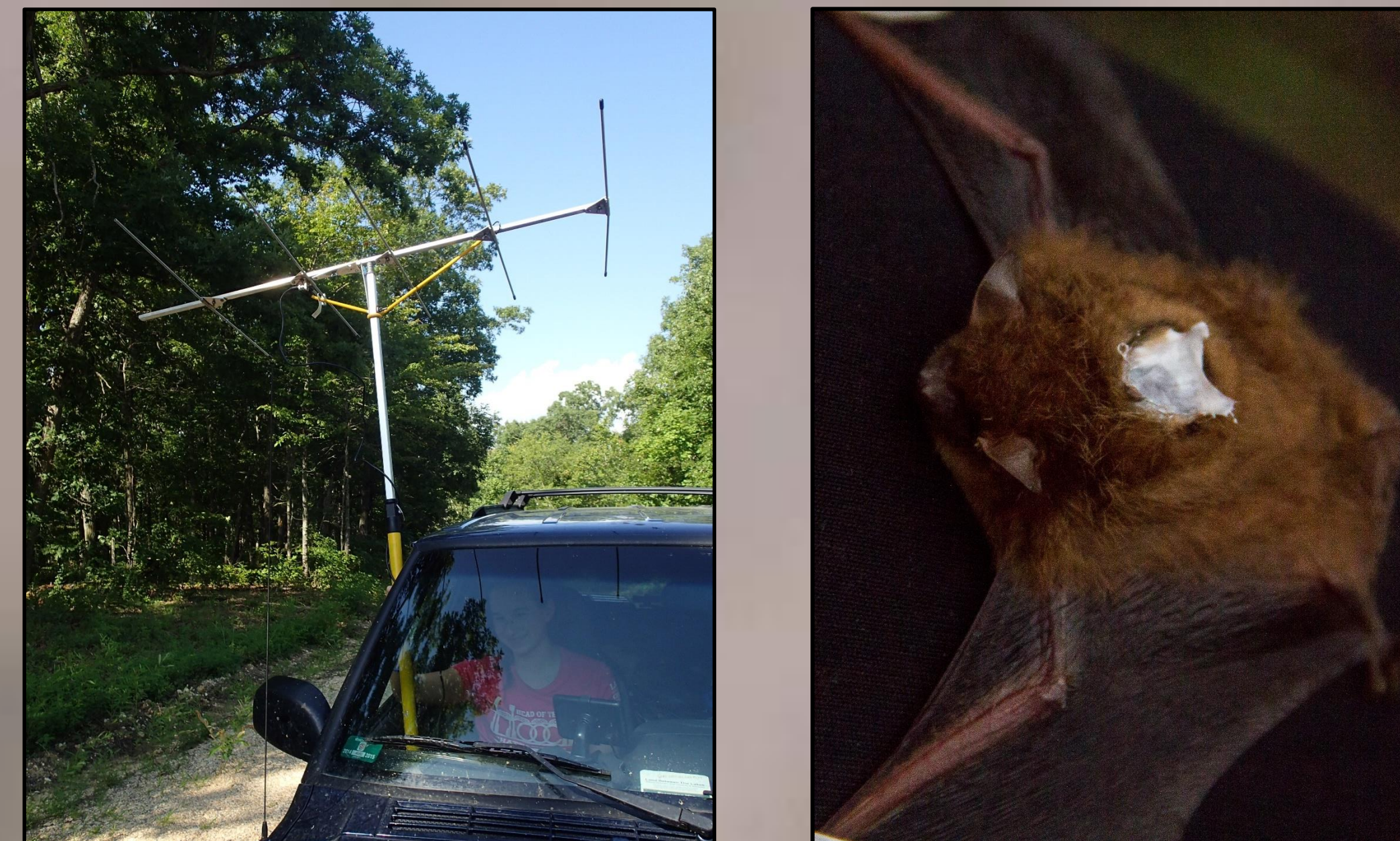
Figure 2. (Left) Five element antenna used in radio telemetry to locate bats. (Right) Tri-colored bat with glue to attach transmitter.
