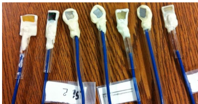
Figure 3.12 Photograph showing \text{GaSb}_x\text{N}_{1-x} electrodes made for photoelectrochemical studies.
