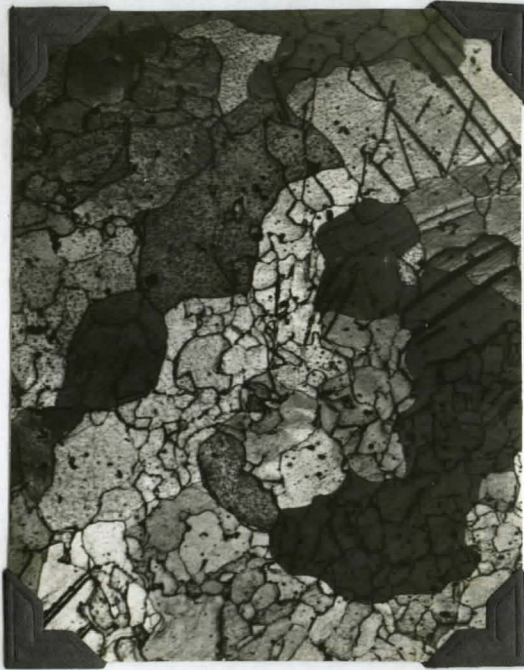
Plate B. After annealing for 1 hour
