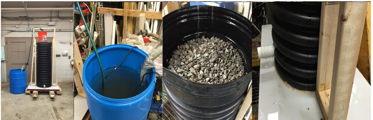
Figure 17-From left to right, the test setup, semi synthetic stormwater runoff, surface of the aggregate layer on top of the column, and the sampling pipe.
