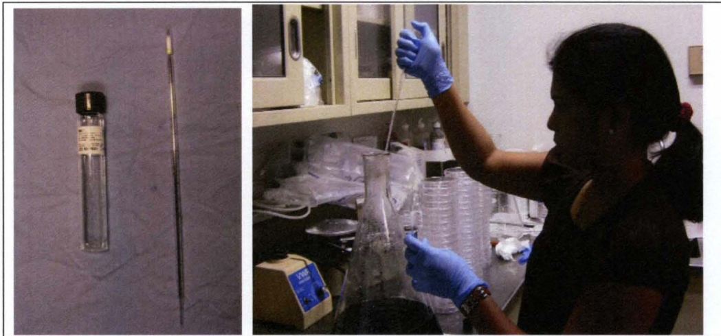
Figure 9. 1% Potassium tellurite pipetted into sterile medium.
