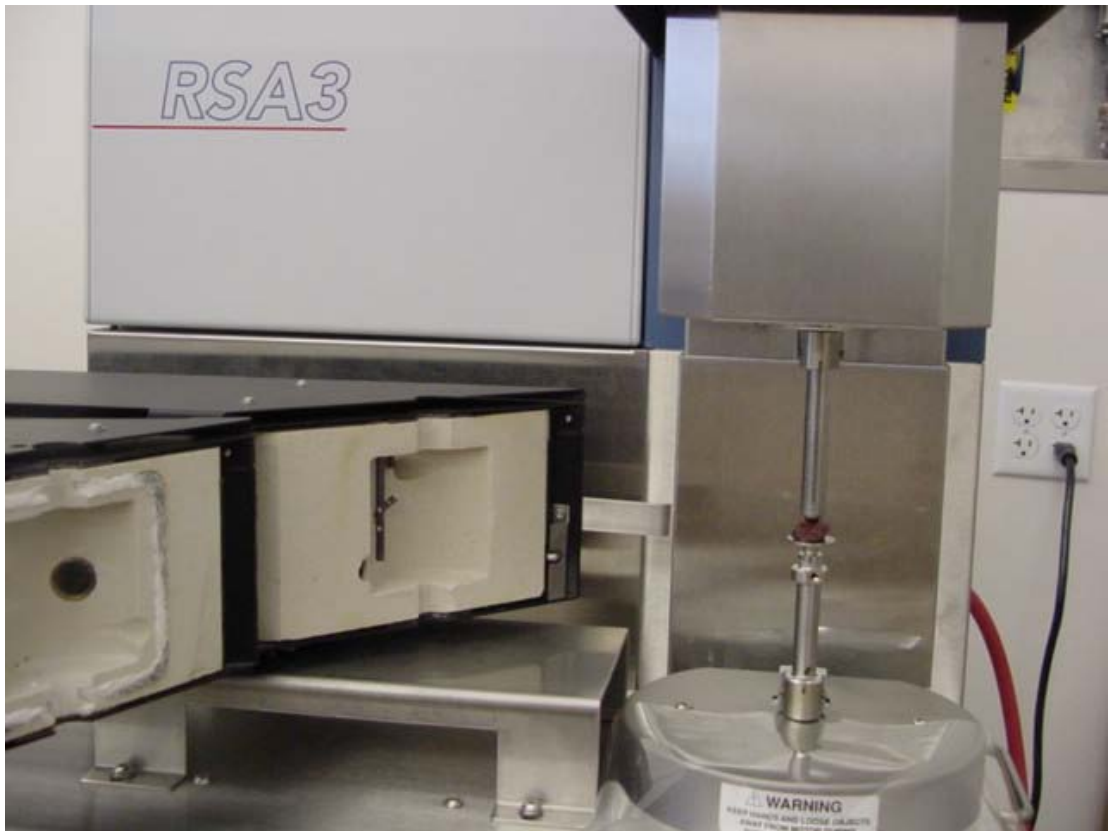
FIGURE 27 – The Dynamic Mechanical Analysis (DMA) machine with RSA3 mode (TA Instruments, Wilmington, DE) from Dr. Roger Bradshaw lab, and the liver tissues for a compression test.
