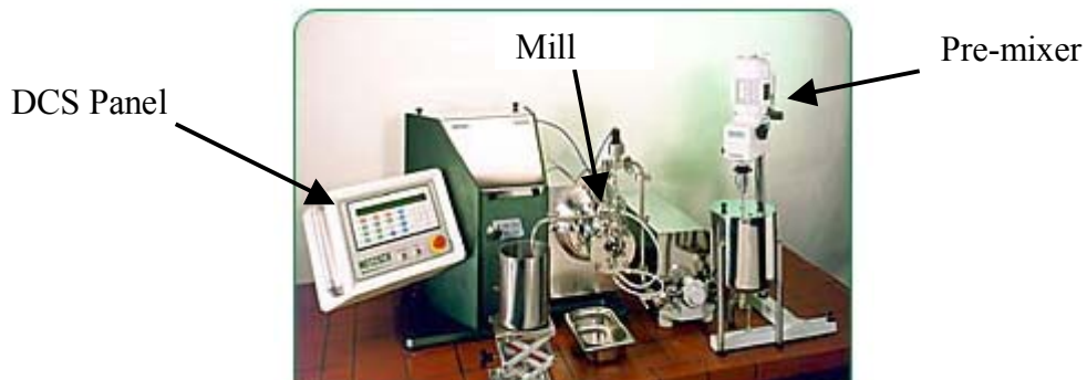
FIGURE 10 –LMZ Labstar Zeta Mill (Netzsch Inc, 2006)
