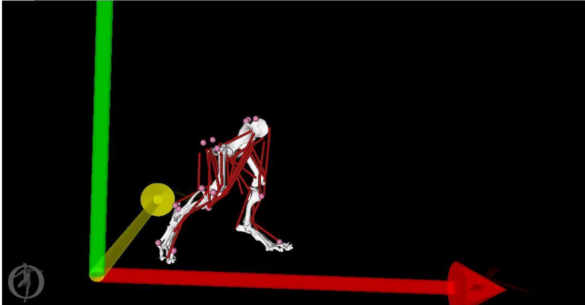
FIGURE 14 - Visualization of the OpenSim pelvic limb model. The model illustrates the bony segments, muscles and motion tracking markers. X-axis is shown in red, Y-axis is shown in yellow, and Z-axis is shown in green. The XY plane is representative of the ground, while gravity acts in the negative Z direction.
