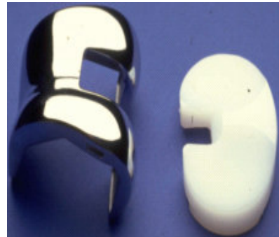
Fig. 3: Knee replacement consisting of a metallic femoral component (left) and UHMWPE tibial component (right) [7]
