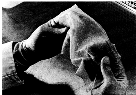
Fig. 8: Artificial skin composed of a layer of silicone rubber and a layer of modified collagen [15]
