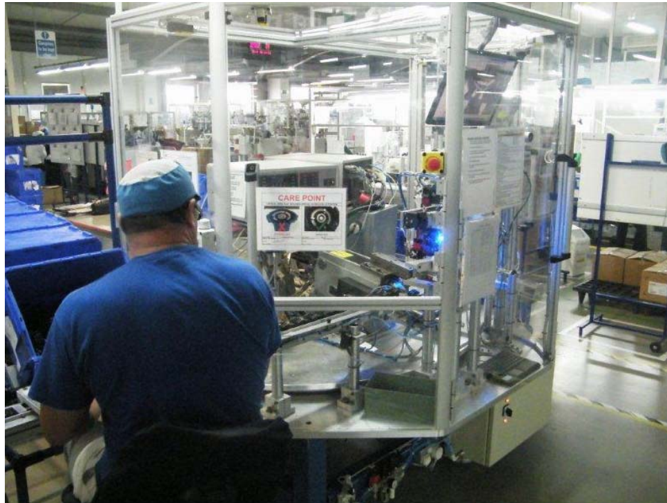
Figure 9. [P2] Ultrasonic Welding.
