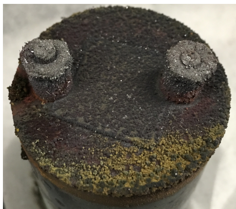
Figure 3.8 – Carbon susceptor with deposition from previous reaction.
