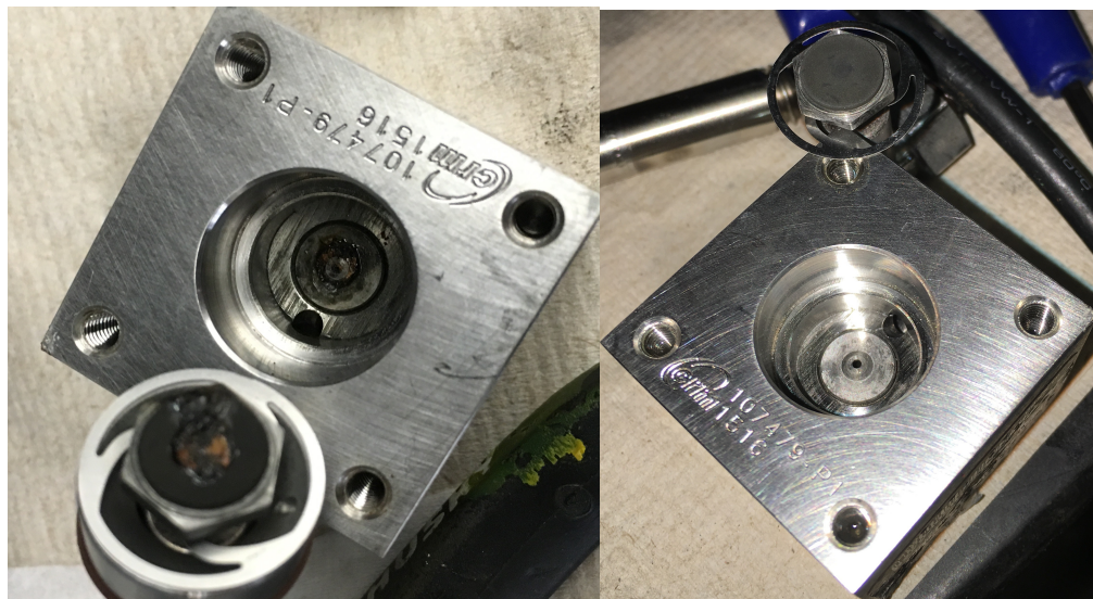
Figure 3.9 Pressure control valve orifice before and after cleaning procedure.
