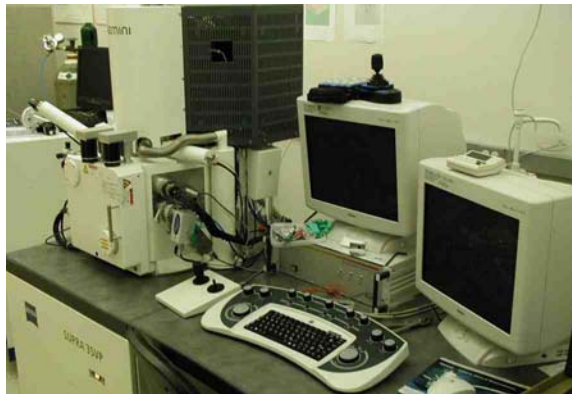
Figure 16. Zeiss SUPRA™ 35VP Scanning Electron Microscope
