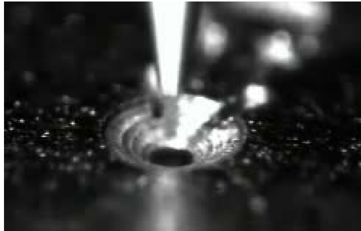
Figure 26. Image of machining process using 150 micrometer endmill in Ti
