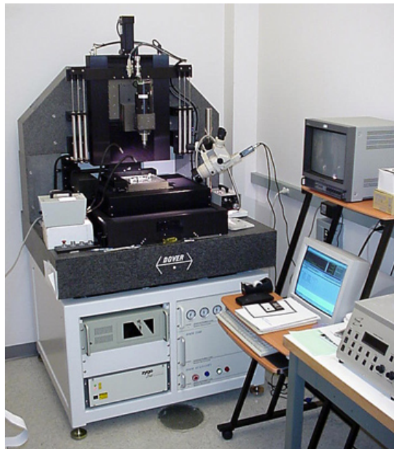
Figure 11. Ultra-High-Precision Micro Milling/Drilling Machine
