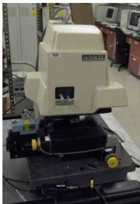
Figure 15. WYKO NT-2000 interferometer
