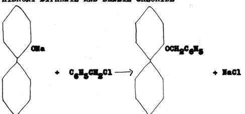
A mixture of 19.2 grams (0.1 mol) of the sodium salt of ortho hydroxy diphenyl and 37.8 grams (0.3 mol) of benzyl chloride was heated in a 200 c.c. round bottom flask connected to a reflux condenser, at a temperature of 176-179°, for 6.5 hours. No reaction was noticeable when benzyl chloride was first added to the ortho salt. The reaction when heated
