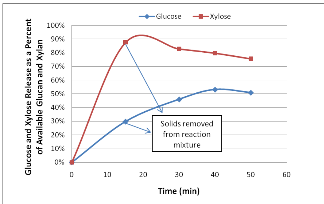
FIGURE 11- Glucose and Xylose Release as a Percentage of Available Glucan or Xylan with Removal of Solids after 15 Minutes
