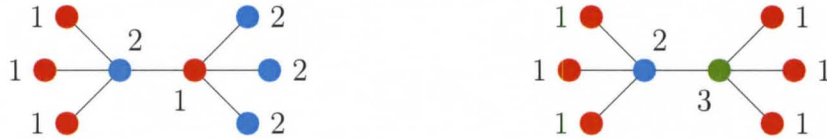
FIGURE 3.2: A graph shown twice, with different colorings. The coloring on the left has weight 12, and uses only \chi = 2 colors. The coloring on the right has weight \Sigma = 11 , but uses 3 colors.
