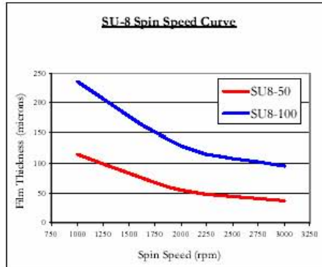
Figure 1. Spin speed vs. thickness curves for selected SU-8 resists.
