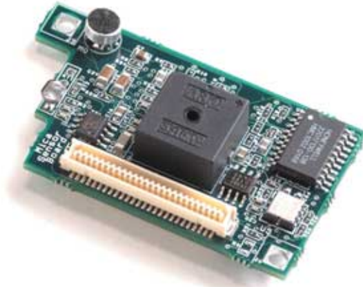
FIGURE 3.2 – XBow Sensor Board with Temperator, Sound, and Light sensors [10]
