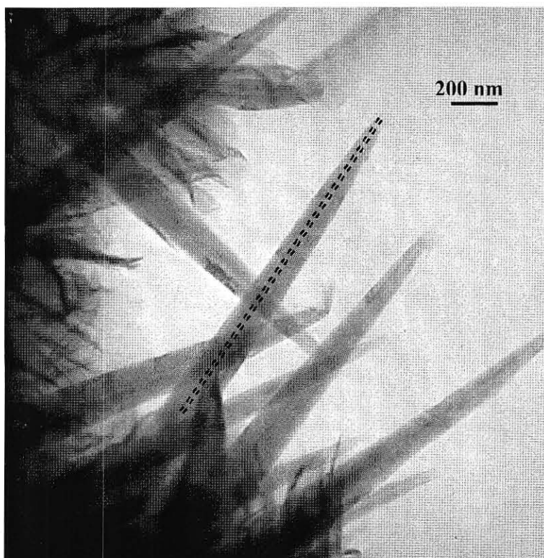
Figure 6.5 Bright field TEM image of the nanopipettes, indicating a hollow core (highlighted, running axially down as indicated).
