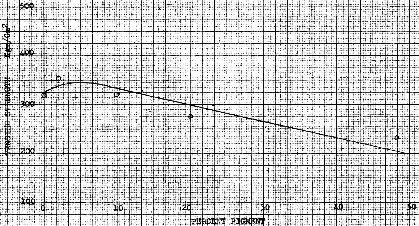
Fig. 12. Variation of tensile strength with percent lithopons
