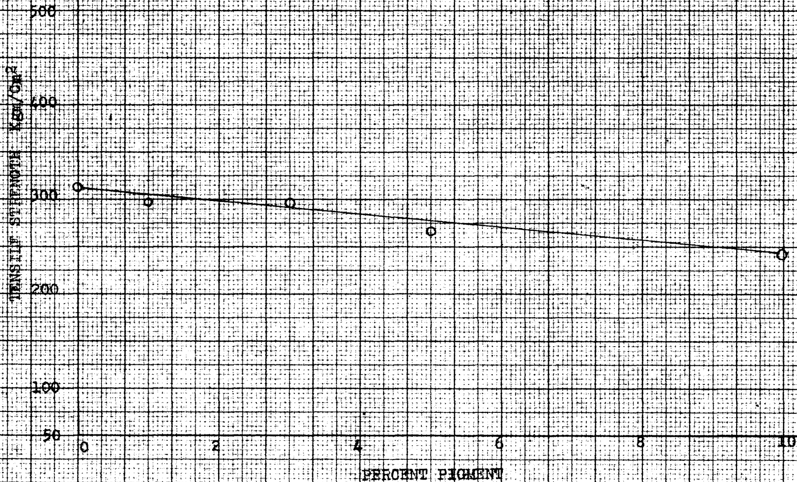
Fig. 14. Variation of tensile strength with percent santocel
