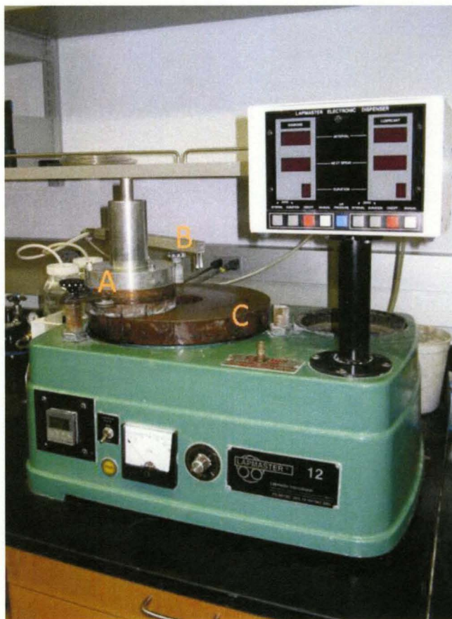
Figure 2-1 Image of Lapmaster Model 12: spindle carrier held in place by yoke (A), slurry dispenser (B), and polishing plate (C).
