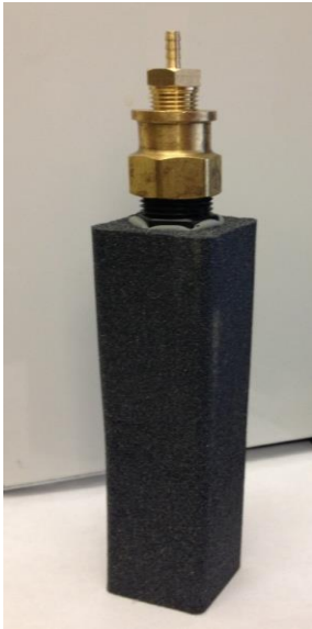
Figure 3-7 Ceramic diffuser used to inject the hydrogen gas
