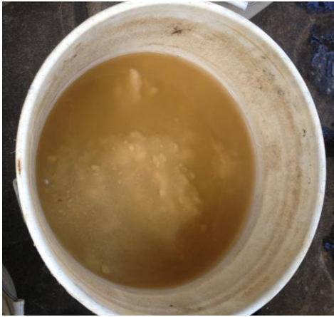
Figure 3-3 Distillery wastewater pulled from production lines, that was provided by a distillery plant located in Louisville, KY, USA.
