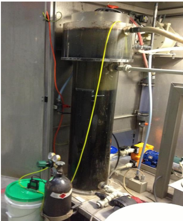
Figure 3-6 Experimental setup to inject the hydrogen gas to the main reactor
